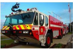
carry a crew of 5 while offering centrally located vehicle controls and displays for improved efficiency. The Titan is powered by the EPA Tier III compliant 665 horsepower Cummins QSX engine combined with an Allison EVS 4800 transmission offering a smooth ride, superior acceleration and reliability. The Titan After a wildfire has been con- holds 1585 gallons of water and 200 gallons of foam. A 1500
